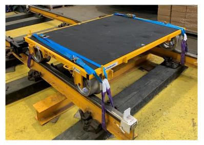
5. Mount the Crane Attachment base to the Type A Trolley, as shown below.
