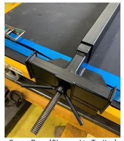
Crane Base (Clamped to Trolley)
