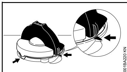
To do this with this STIHL cap, raise the grip on the top of the cap until it is upright at a 90° angle. Insert the cap in the fuel
