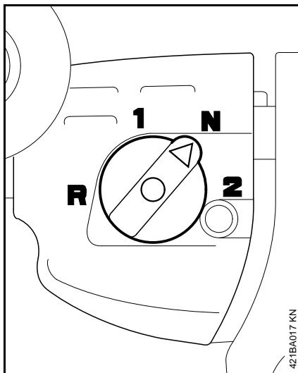
The power drill is equipped with a change-speed gearbox. Depending on the application and the drilling tool used, the speed can be adjusted to suit requirements.
