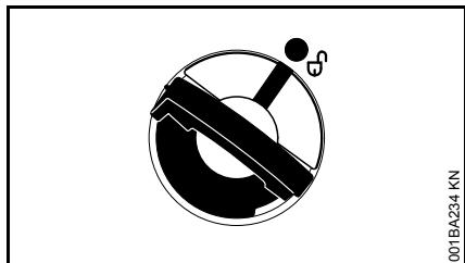
Markings on filler cap and housing must align.
