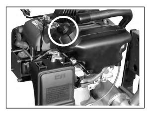
• If the motor is cold, position cold start indicator to 1 o 1.
