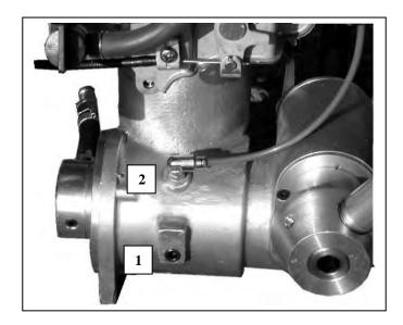
To check the gearbox oil level. Remove the oil level plug (1) and check that the oil level is up to the level of the bottom of the threaded hole. If not, remove the vent pipe plug (2) and fill with Renogear V220EP (or equivalent). The open end of the vent pipe is located within the lifting handle and should always be replaced in this position after filling. Replace both plugs before use.
