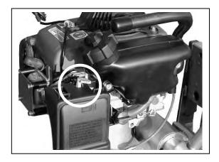
• Rotate the fuel cut off valve to the horizontal position.
