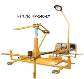
The unit has easy to change drill guides and bits, easy to adjust depth stops/apply lever assisted hand feed/ and drill depth stop.
