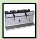
To ensure that the holes are correctly distanced from centre to centre, a hole centre location unit is available which fits on top of the rail and can quickly be secured by tightening two handles. Recesses in the plate are designed to accommodate the machine as it is lowered into position. These features provide complete accuracy when working in difficult and low light conditions.
