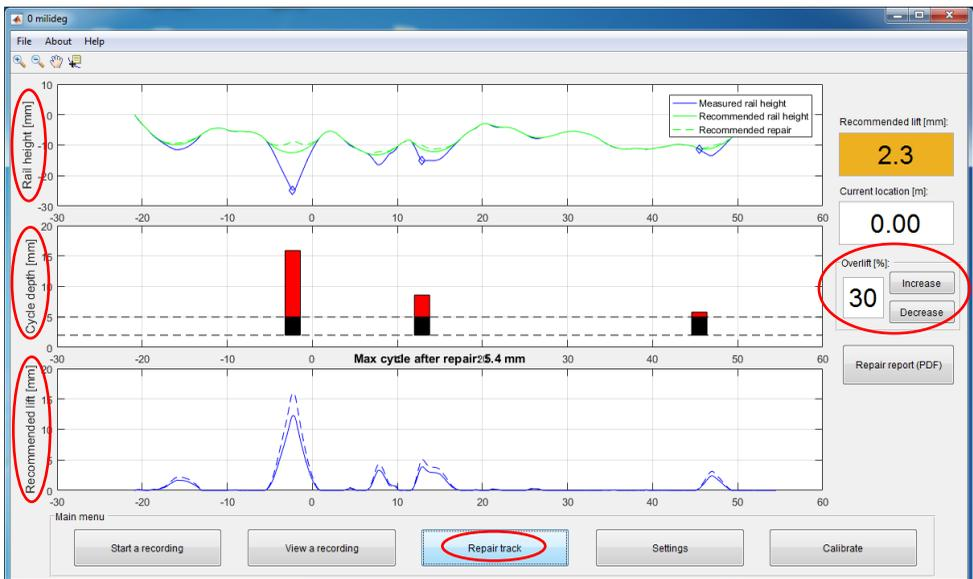
**Figure 31: Repair Track - Overlift at 30%**
