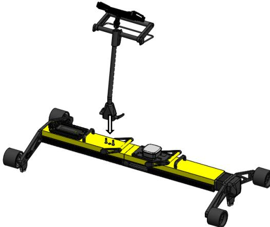
**Figure 6: Handle Assembly Step 1**
