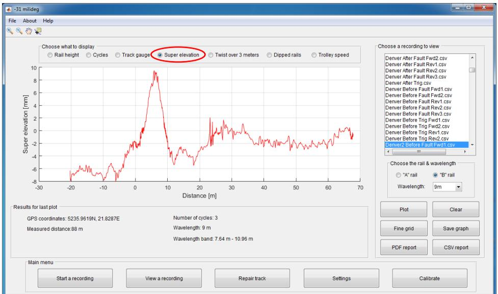
**Figure 25: Plot of super elevation**
