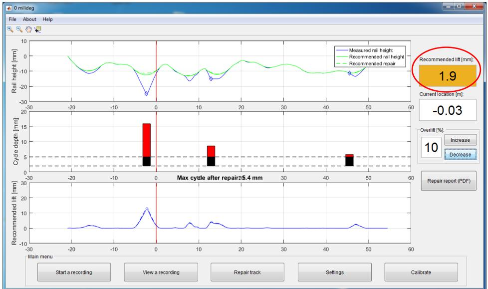
**Figure 33: Repair Track - Overlift at 10%**
