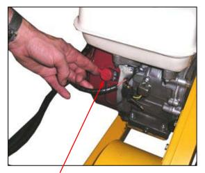
Turn the engine **on/off** switch to the **on** position.
