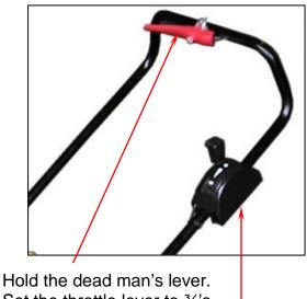
Set the throttle lever to <sup>3</sup>/<sub>4</sub>'s. – Pull the engine start cord sharply.
