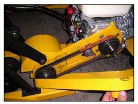
Remove the guard to expose the drive belt to check for excessive play
