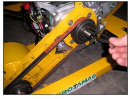
Screw the grubscrews into the jacking holes to release the taper-lock bush
