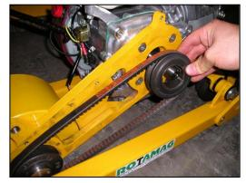
Remove the taper-lock bush and replace the belt. Re-fitting is a reversal of this procedure
