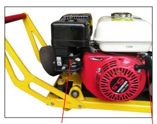
Push the fuel switch to the **on** position. If starting the engine from cold push the choke lever to the **on** position. (Located above the fuel switch)
