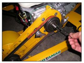
Remove the two grubscrews retaining the taper-lock bush on the drive pulley
