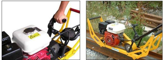
Increase the speed of the engine to normal running speed by moving the throttle to the "hare" position. Move the brush operating lever to the forward position to allow the wheel to come into contact with the rail head.
