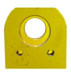
Check hole threads and hexagon set pins for the top load pin location plate.
