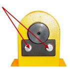
Check the clamp body side plates are not bent and are parallel.
