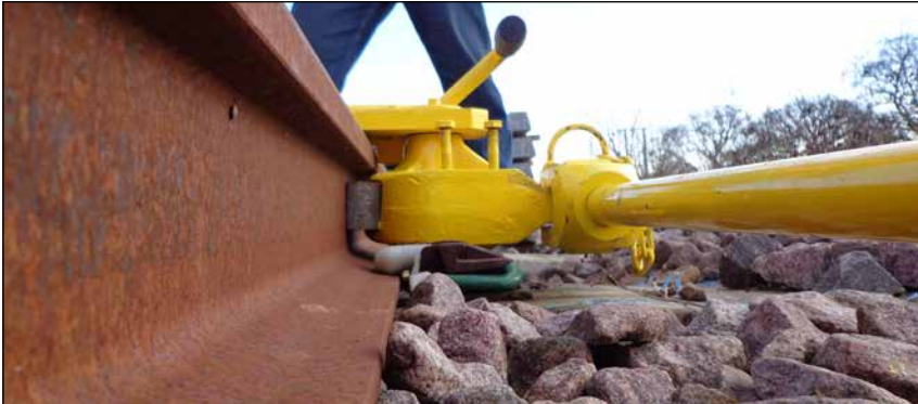
▼ RP70 Rail Puller in an obstructionless pull.
