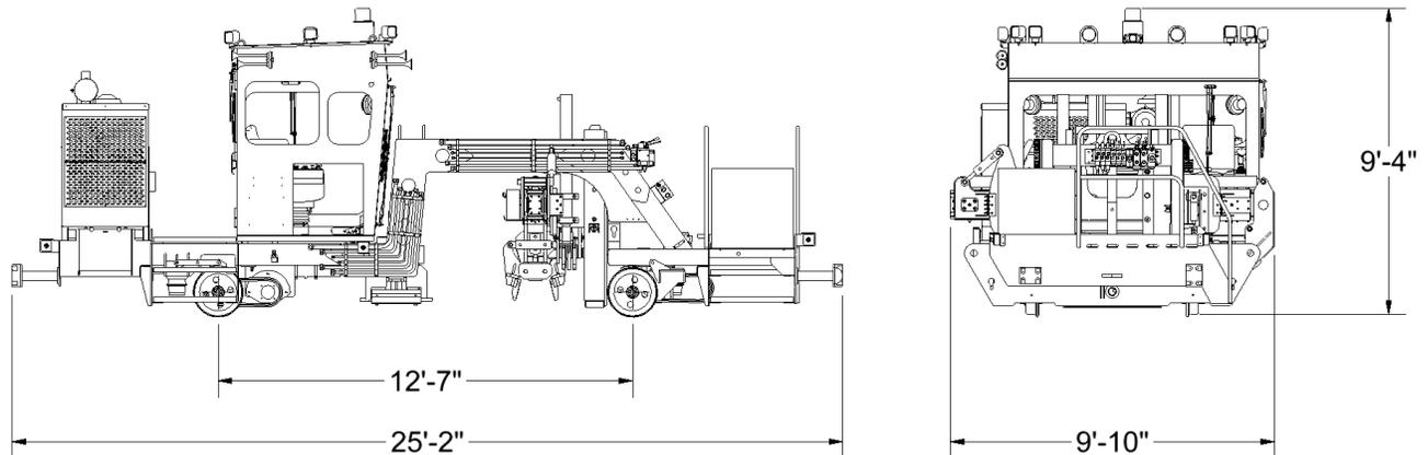
Knox Kershaw's KTR450 Tie Replacer is an operator-friendly low-maintenance machine capable of removing and inserting ties (timber and concrete). The 88"-stroke workhead generates extraction forces exceeding 23,000 lbs. A wide offset cab gives the operator full view of the workhead and ties.
