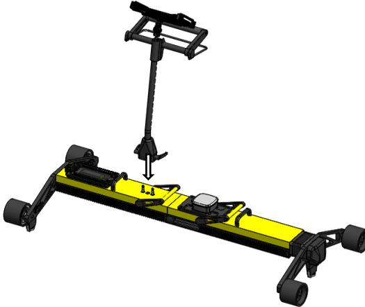
**Figure 6: Handle Assembly Step 1**
